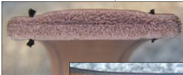
Above: cross-section shows construction of 5-Shot Leather belt. Right: Stitching and skiving gives belt dressy look.
