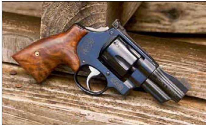
Custom revolver work by Grant Cunningham includes a bobbed hammer with the single action notch removed.
