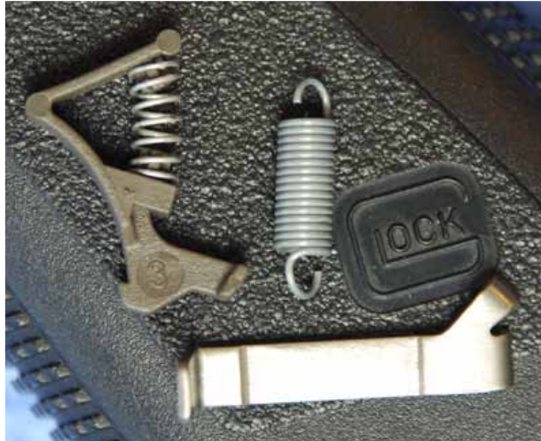
Glock's New York trigger (left) shown with standard trigger spring and connector.
