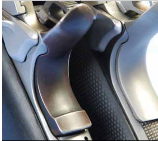
Most 1911 pistols made today have grip safeties with a memory bump as shown on the left.
