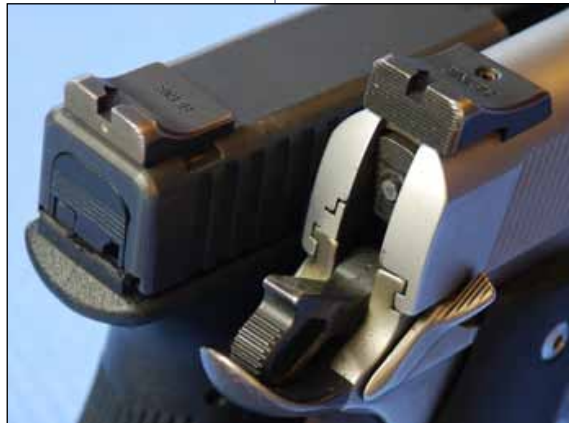
Heinie Straight Eight night sights (left) and standard match grade sights (right).
